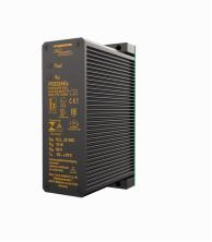
The PSD24Ex module supplies the excom® system with power to the full extension. The module rack is designed in a combined protection rating of Ex m, Ex e and Ex i and can therefore be used in zone 1. It is also fully potted and installed in a die-cast aluminium frame.
