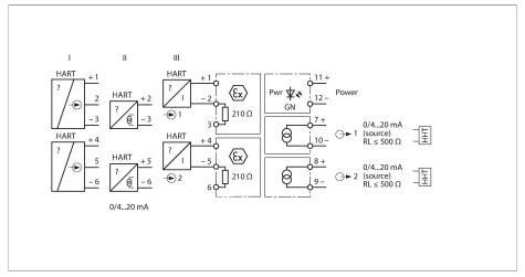
The 2-channel HART isolating transducer IM33-22EX- The removable terminal blocks feature test HI/24VDC is designed to operate intrinsically safe HART 2-wire transducers (III) in the Ex area and to transmit the measured signals to the non-Ex area. In addition to the analog signals, also the digital HART communication signals can be transmitted bidirectionally.
