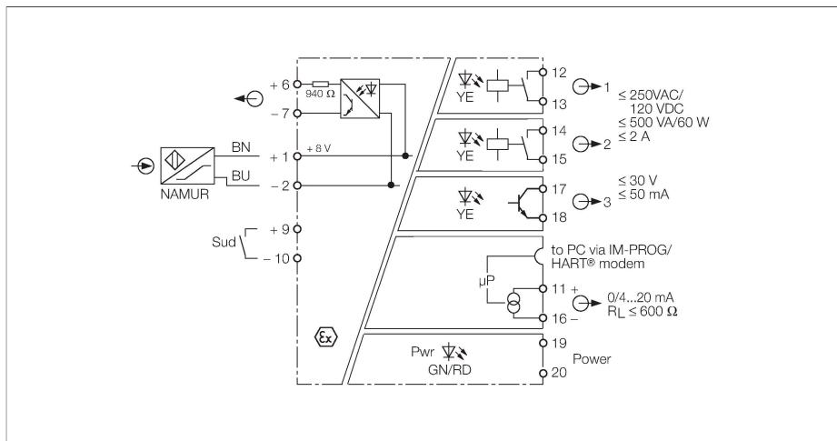
The rotation speed monitor IM21-14EX-CDTRI monitors frequencies, rotation speeds and pulse trains of rotating motor, gear or turbine parts according to over or undershoot of adjusted limit values. The current value is indicated on a display on the front of the device.
