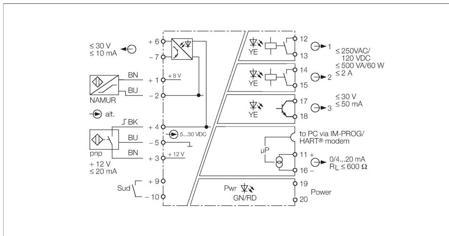
The rotation speed monitor IM21-14-CDTRI analyses frequencies, rotation speeds and pulse trains of rotating motor, gear or turbine parts according to over or undershoot of adjusted limit values. The current value is indicated on a display on the front of the device.
