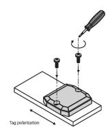
3M 300 LSE adhesive tape (ideal temperature for application: 21–38 °C). Any silicone sealing compound with a maximum thickness of 2 mm between the metal surface and the underside of the tag. M4 screws Rivets (diameter: 4 mm)
