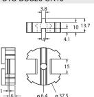
Spacer for dual sensor actuation kitBTS-DSC26-EB20
