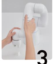
The main unit weighs approximately 4 kg providing easy portability, and offers a load capacity of 500 g. The integrated controller not only reduces wiring, but also allows consolidated control with other devices. ORIN is supported as standard.
