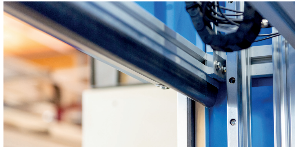
The Mayser safety edge ensures accidents to personnel are prevented at the special-purpose machine.
